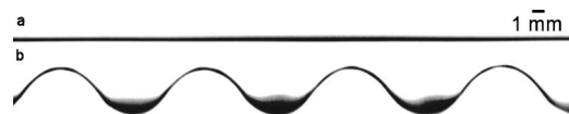
FIG. 2. Images of the straight morphology (a) observed in the prebifurcation branch and pattern-forming (b) present in the post-bifurcation branch. In both images the air is located above the interface and silicon oil is located below the interface. Experiment running at b_o=400 \mu\text{m} and \omega=4.85 \text{ rad/s} (a) and \omega=5.39 \text{ rad/s} (b).
